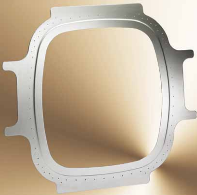
fuselage frame Airbus A350 aluminium 7050 T7452 2,410 x 500 mm | 330.0 kg
