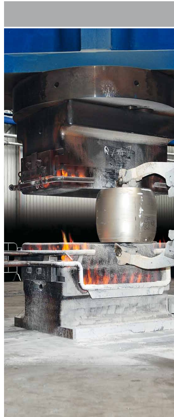
forged truck wheel aluminium EN AW 6082 22.5J x 11.75 | ET 0 | 26.0 kg
